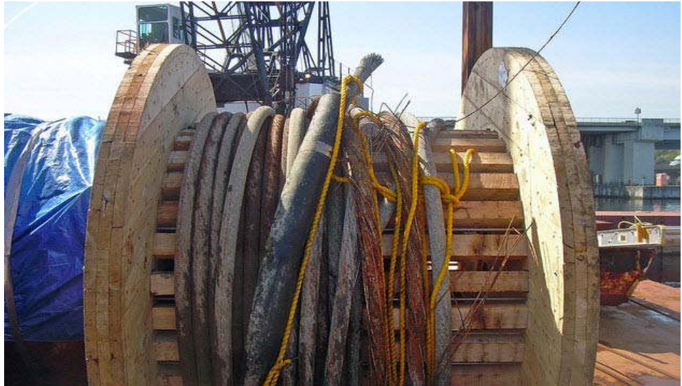
Figure 16.3.18 Frayed Cables Removed from a Floating Bridge
