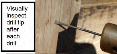
Visually inspect drill tip after each drill.
