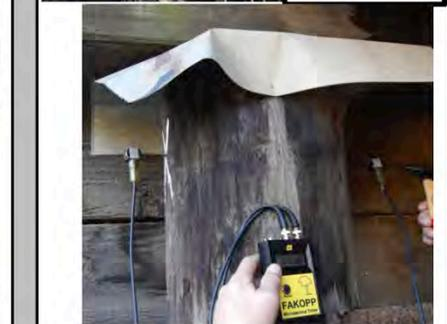
Typical areas of concern are below the cap, at water line and slightly below water line. Waterproof transducers are available.
