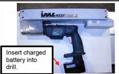
Insert charged battery into drill.
