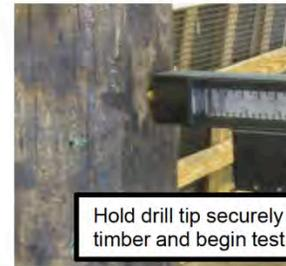
Hold drill tip securely against timber and begin testing
