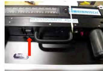
Turn on the unit by pressing the switch on the underside.
