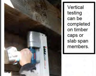
Vertical testing can be completed on timber caps or slab span members.
