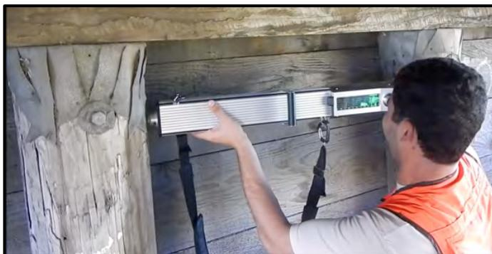
Figure 6.6. Electronic display on a resistance drill.
