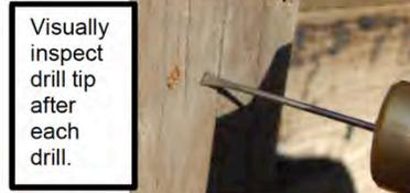
Visually inspect drill tip after each drill.
