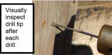
Visually inspect drill tip after each drill.
