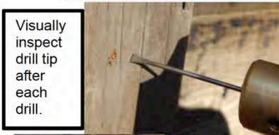
Visually inspect drill tip after each drill.
