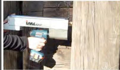
Resistance drilling can be used independently or to confirm stress wave testing results.
