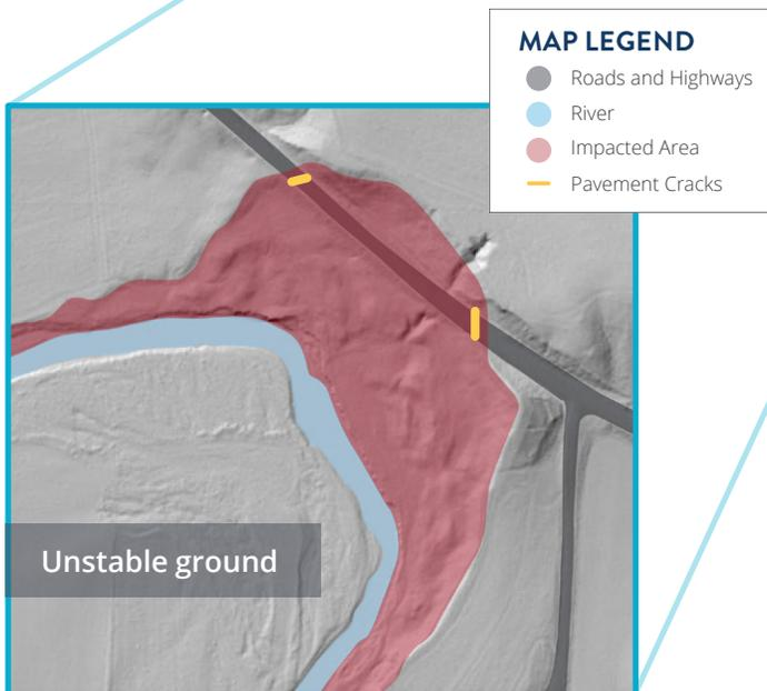
The illustration below highlights findings of this analysis – a lot of the ground underneath the roadway is unstable. Repairing the roadway in place would require significant specialized construction to stabilize the ground.
