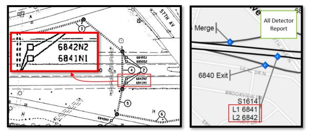
Figure 3-27: Loop Detector Function Designations
