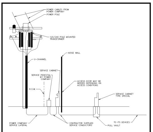
Figure 3-3: Typical Power Service - Pole-Mounted Transformer behind Noise Wall
