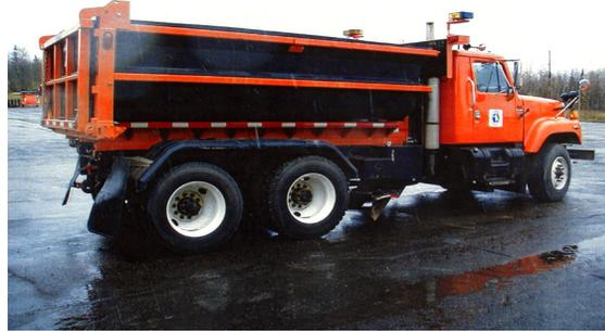
**Background:** The standard steel truck bodies require maintenance in painting, rust and dent repair, and also because of the type of rock in this area they become dented. This does not permit materials to slide out freely when dumping and especially during sanding operations.
