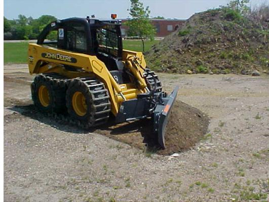
**Background:** Skid steers are a valuable piece of equipment to maintenance crews everywhere in state. These units are in many cases, the backbone of the maintenance workers arsenal of equipment. They perform a huge variety of tasks that would otherwise have to be accomplished manually resulting in a great reduction in hours of labor and lighter duty equipment.
