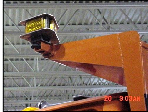
**Background:** LED Emergency Lights are becoming more common on trucks and other equipment in the maintenance and construction fields. These new systems do have advantages in that they last much longer and also use a very low amount of electrical current to operate. With Mn/DOT trucks already drawing close to the maximum amperage output this can be extremely beneficial in reducing alternator and other electrical problems producing a substantial reduction in shop time and repairs.
