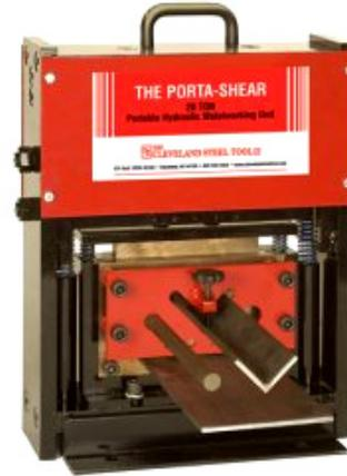
**Background:** When working in the field fabrication of steel railings and other components can be difficult. Clean straight lines of cut ease fabrication by providing a better fit. This then requires less welding time and a better-finished product is achieved.
