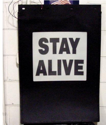
**Background:** Many new ideas in safety lighting are introduced each year. Electroluminescence technology has been applied to Stay Back Stay Alive signs and lighted mud flaps. These will be mounted low to the ground to increase visibility of Mn/DOT trucks during plowing operations. Many times snow is lifted up when plowing resulting in snow clouds. The lighted mud flaps hopefully will allow approaching motorists an increased view of the truck under these adverse conditions.
