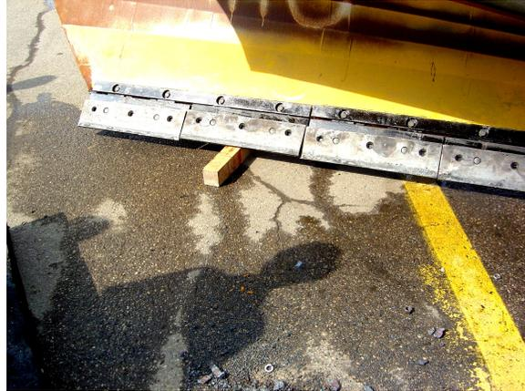
**Background:** Carbide cutting edges are expensive but a necessity for Mn/DOT to accomplish an effective plowing operation. Much time is spent installing new carbide edges as well as other costs in hardware and materials. Longevity of carbide edges is crucial in keeping costs to a minimum.
