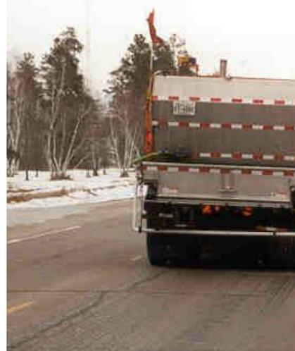
**Background:** Previous research has shown that a driving condition exists during fog that affects motorists in a negative way. Speeds are actually increased rather than decreased relating to a hazardous condition. Also during plowing operations these conditions are closely repeated by snow clouds associated with that type of work. The term for this is low luminance contrast.
