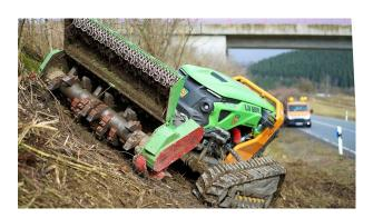
**Project Description:** Roadside maintenance crews often mow in wet areas and on steep banks, situations vulnerable to rutting and to rollovers and other accidents that threaten crew safety. Green Climber mowers feature wide bases, weight-distributing track systems and low centers of gravity much less likely to cause damage or to roll over, and remotecontrol operation that keeps crews out of harm's way.
