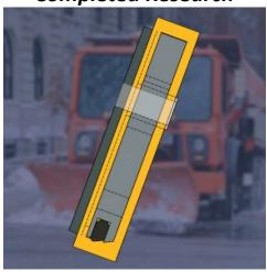
**Project Description:** Cutting edges on snowplow blades require more frequent replacement than other snowplow parts. Thicker and stiffer blades with a one-piece design should require fewer removals and installations and be more durable and cost-effective.
