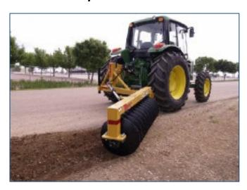
**Project Description:** Road shoulder problems can quickly undermine the road foundation. The shoulder reclaimer is a claw attachment that is used to fill in ruts and smooth the shoulder. The unit currently in use is mounted on the right side of the tractor and can only be used on that side. The Tiger Claw model is positioned in the middle of the tractor for transport and can be used on either side.
