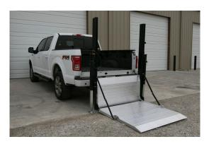
**Project Description:** Road maintenance crews use trucks to move equipment and supplies to and from job sites and other shops. A new lift gate will reduce hand-lifting and moving heavy items during busy maintenance periods when other lift gates are unavailable.
