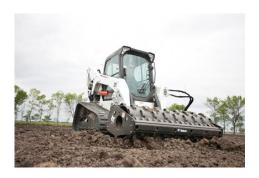
**Project Description:** Culvert repair requires a range of heavy equipment, including tools for compacting soil effectively to ensure culvert stability and performance. Maintenance crews can use these new rollers as attachments to a single vehicle to respond promptly and efficiently to urgent and routine stormwater management needs.
