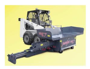
**Project Description:** Paving around certain structures and small areas can be difficult and time consuming. Oftentimes, small paving jobs require manual labor which adds time and costs to a project. Mini pavers can maneuver around tight spaces on smaller worksites such as sidewalks, wheel ruts, edge drop offs, utility trenches and driveways.
