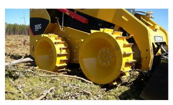
**Project Description:** Ribbed all-steel wheels were mounted on forestry equipment to resist tearing that was being experienced by rubber tires or logging tracks when driving over abrasive debris while grinding trees.
