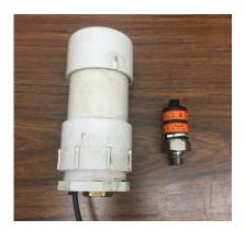
**Project Description:** Up/down snowplow sensors allow snowplow operators and managers to track mileage of use and wear on plows and cuttingedges, one of the most commonly replaced snowplow parts. Sensor data can be used to determine the most effective cutting edges for various types of plow and pavement types.
