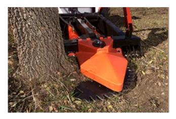
**Project Description:** Removing small trees from rights of way, ditches and other roadside terrain can be time-consuming and difficult. Chain saw work, especially during inclement weather, can be a dangerous use of manpower. A boom-mounted saw attachment for heavy equipment may offer a solution.
