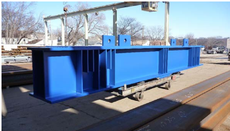
The 500 ton main jacking beam is awaiting delivery to MnDOT
