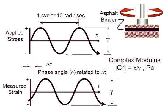
Figure 4.5. DSR Test Schematic (9)
