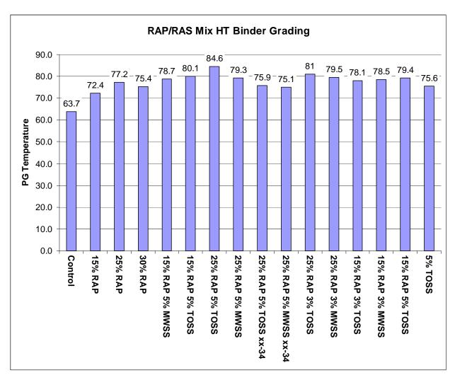
Figure 4.1. RAP/RAS Mixture High Temperature PG Binder Grading
