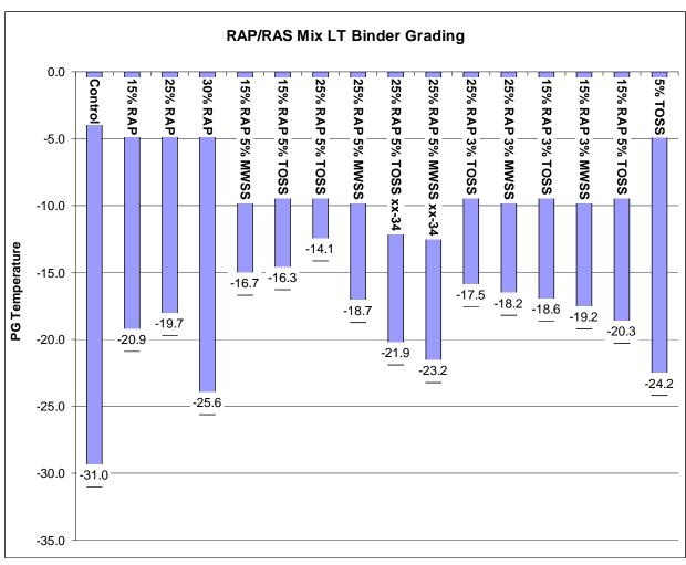
Figure 4.2. RAP/RAS Mixture Low Temperature PG Binder Grading
