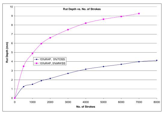
Figure 4.34. Rut Depth vs. No. of Strokes for Mixes 5 & 6 (Shingle Type @ 5 & 15% RAP)
