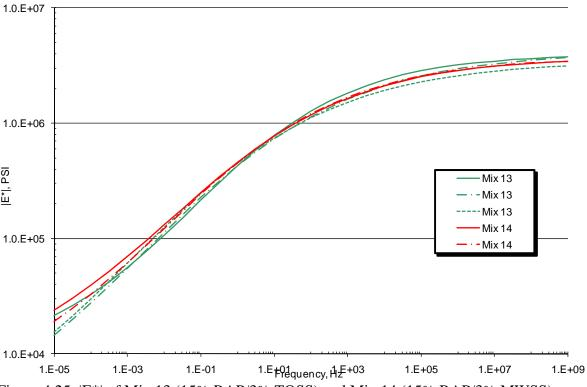
Figure 4.25. |E\*| of Mix 13 (15% RAP/3% TOSS) and Mix 14 (15% RAP/3% MWSS)
