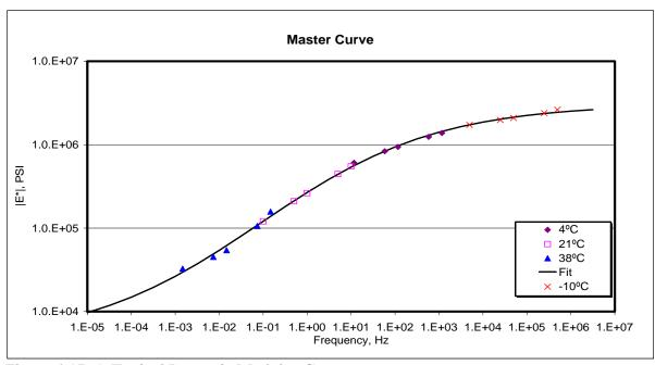
Figure 4.17. A Typical Dynamic Modulus Curve
