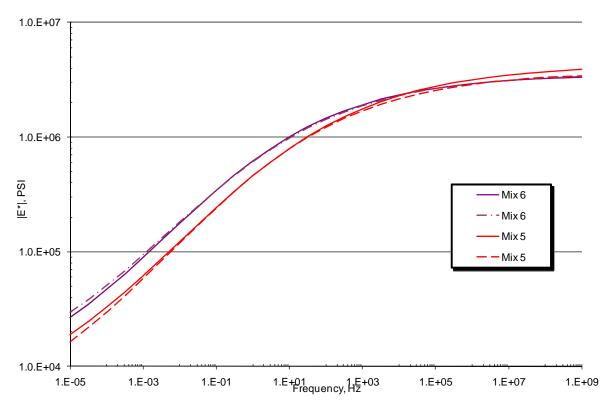
Figure 4.21. |E\*| of Mix 5 (15% RAP/5% MWSS) and Mix 6 (15% RAP/5% TOSS)
