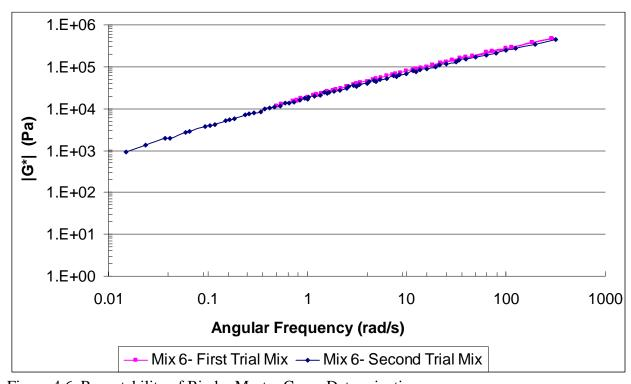
Figure 4.6. Repeatability of Binder Master Curve Determination
