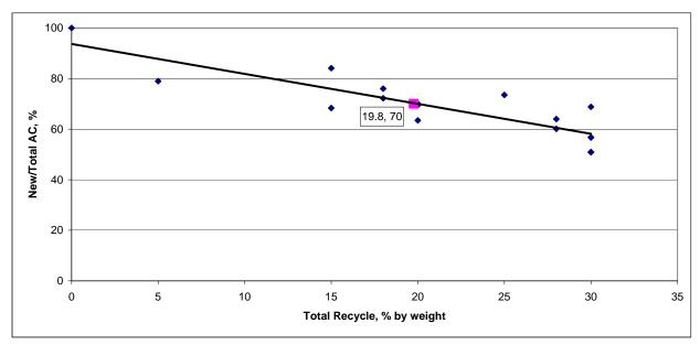
Figure 3.5. New Binder to Total Binder Ratio vs. Total Recycled Materials Content
