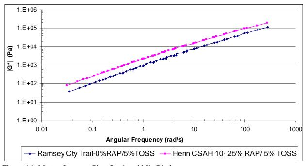
Figure 4.9. Master Curve on Plant Produced Mix Binders
