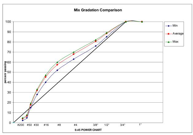
Figure 3.4. Mixture Design Gradations
