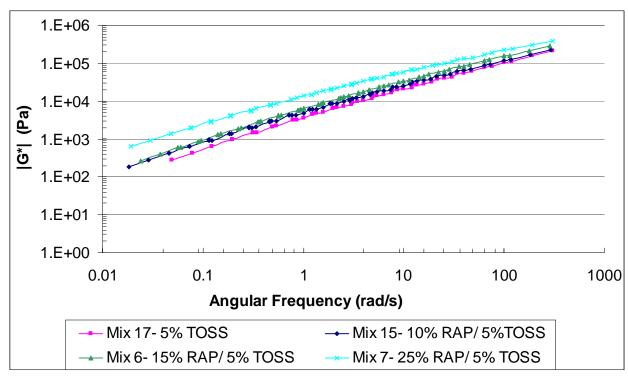
Figure 4.11. 5% TOSS Mixtures with Increasing RAP
