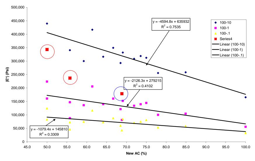
Figure 4.28. |E\*| vs. % New AC at 100 °F
