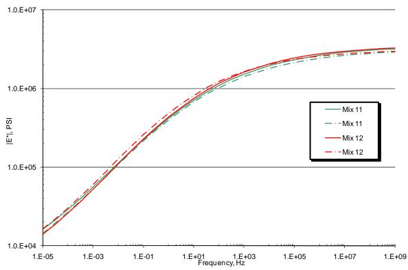
Figure 4.24. |E\*| of Mix 11 (25% RAP/3% TOSS) and Mix 12 (25% RAP/3% MWSS)
