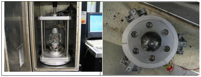
Figure 4.16. Dynamic Modulus Testing Apparatus and LVDT Setup
