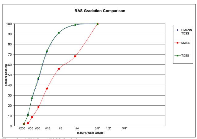
Figure 3.1. MWSS and TOSS Gradations
