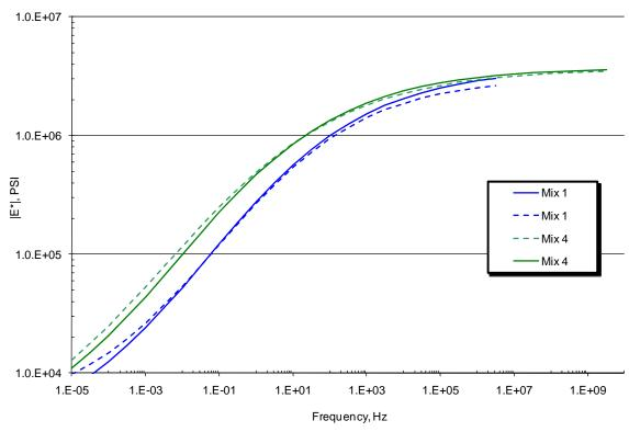
Figure 4.18. RAP Effects on |E\*| Mix 1 (Control) and Mix 4 (30% RAP)
