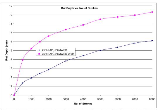
Figure 4.35. Rut Depth vs. No. of Strokes for Mixes 8 & 10 (Effect of -34 Binder)
