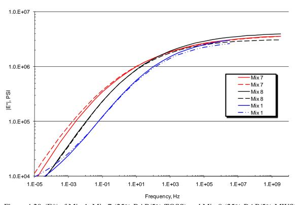
Figure 4.20. |E\*| of Mix 1, Mix 7 (25% RAP/5% TOSS) and Mix 8 (25% RAP/5% MWSS)
