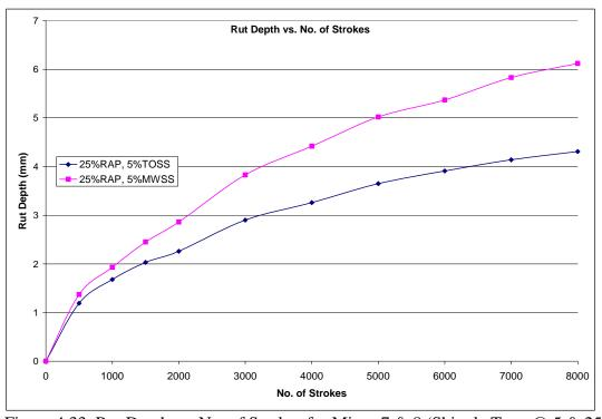
Figure 4.33. Rut Depth vs. No. of Strokes for Mixes 7 & 8 (Shingle Type @ 5 & 25% RAP)
