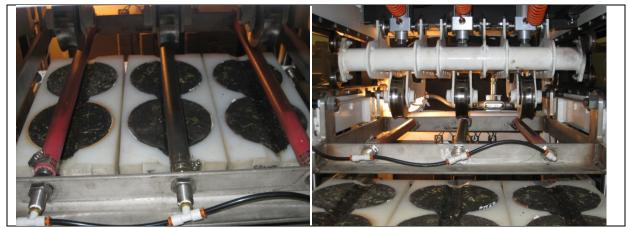
Figure 4.31. Asphalt Pavement Analyzer (APA) or Rut Tester
