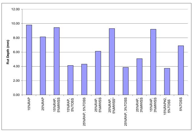
Figure 4.32. Rut Depth after 8,000 Strokes
