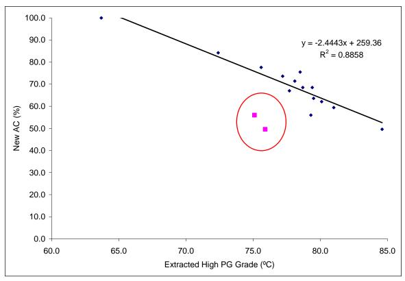
Figure 4.4. New Binder to Total Binder Ratio vs. High Temperature PG Grade
