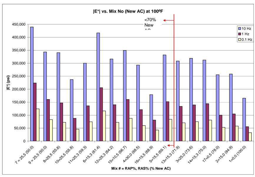
Figure 4.27.  $|E^*|$  vs. Mix No. at 100 °F
