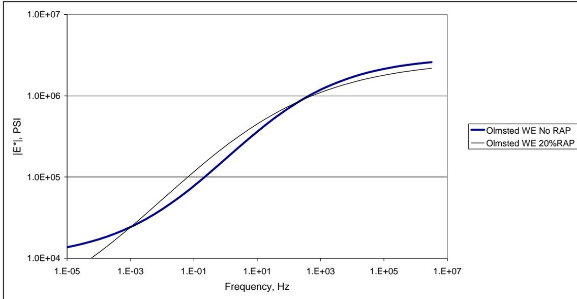
**Figure 26 –  $|E^*|$  master curve for Olmsted CR 112 wear course specimens; 58-34.**
