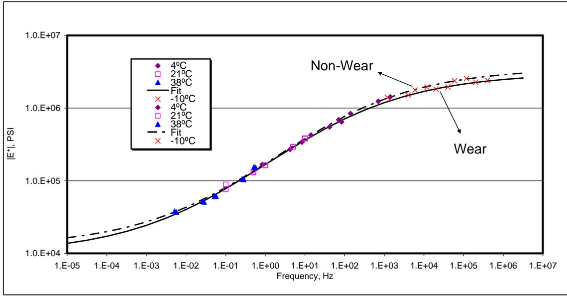
**Figure 24 –  $|E^*|$  master curve for Olmsted CR 112 wear and non-wear course specimens; 58-34 with no RAP.**
