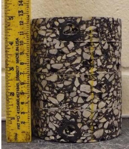
**Figure 16 – Wear course |E\*| specimen from Olmsted CR 112 cores.**
