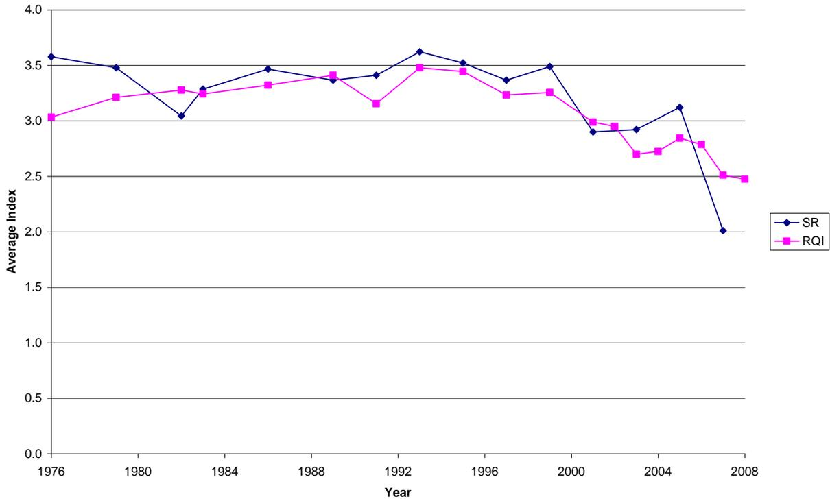
Figure 3.5. Average Pavement Condition Prior to Overlay
