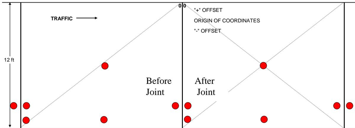
Figure 4.1. Routine FWD Testing Locations in Test Cell 53-1
