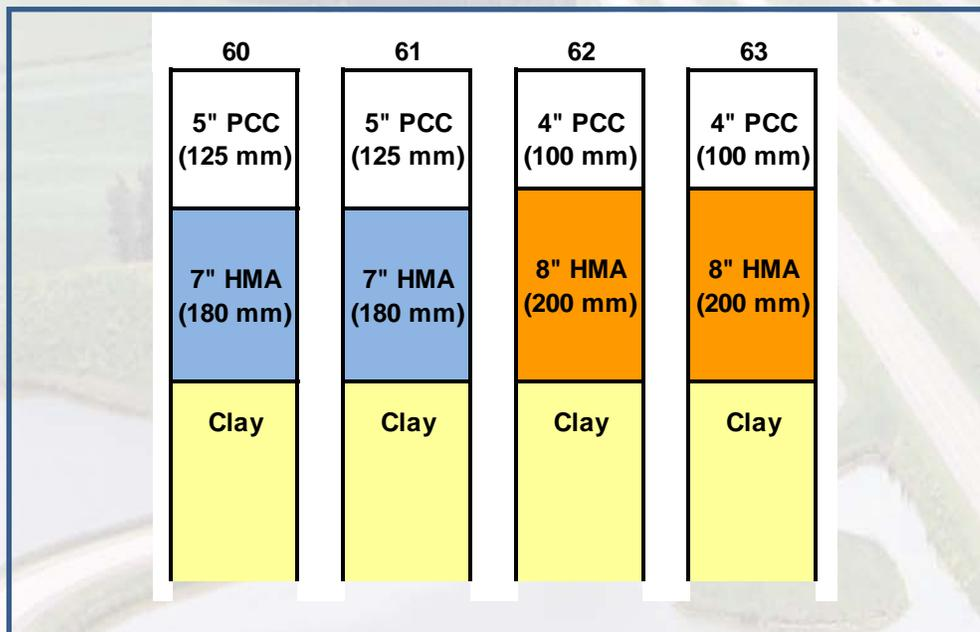
Figure 2. Design details for MnROAD whitetopping test cells 60-63.
