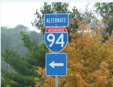
Permanent alternate route signs use the Interstate shield to keep diverted drivers on track.
