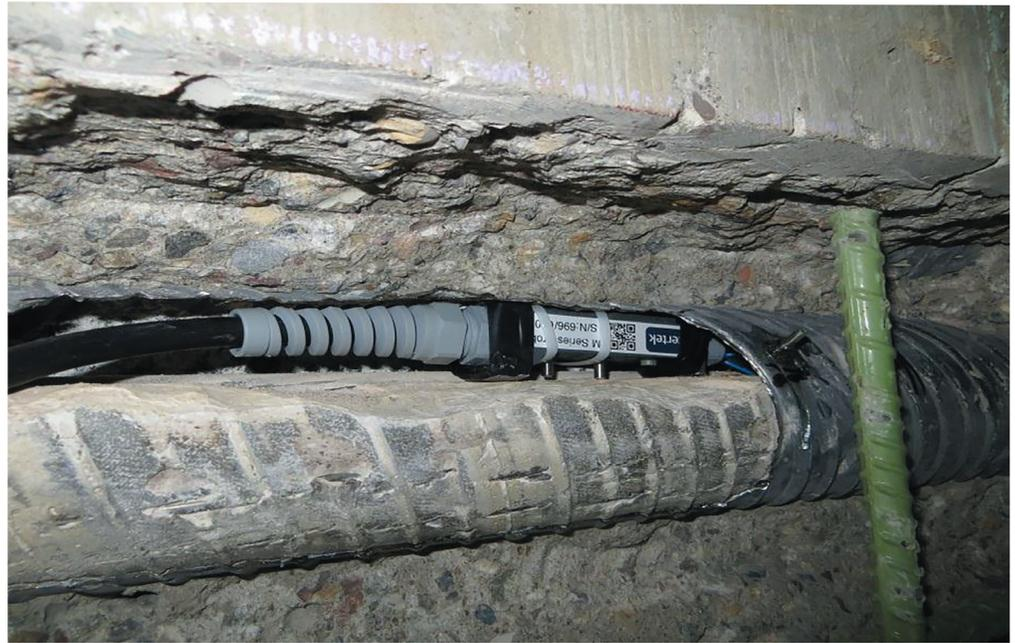
Researchers installed corrosion-monitoring sensors within grout voids at two locations. Measurements are taken manually using a handheld data collection unit and patch cable.
