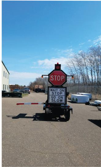
The final device delivered to MnDOT offers large electronic signage, lights and a traffic bar on a movable platform. The unit is easily visible to road users and can be operated remotely from a safe distance off the roadway.
