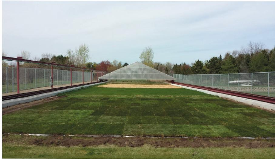
This automatic rain shelter carefully controls the irrigation of test areas, moving to protect the trial areas when it senses rain and moving away from the trial plots when rain ends.
