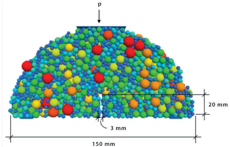
Researchers developed a computer model of SCB tests that can be used to infer the properties of asphalt mixture binders using inputs from the less-expensive BBR test.
