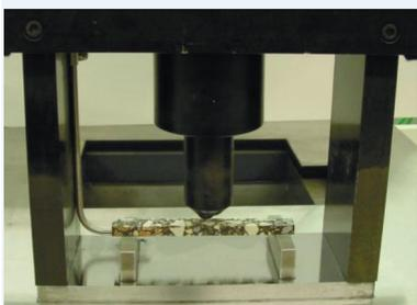
Although simpler and less expensive than an SCB test, a BBR test only evaluates the properties of a mixture's coarse aggregates.
