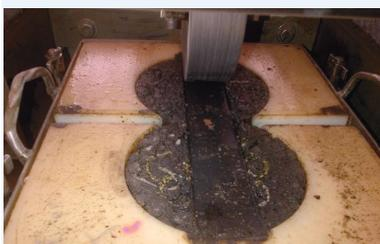
The Hamburg wheel track test assesses an asphalt mixture's rutting resistance and may be used in BMD.
