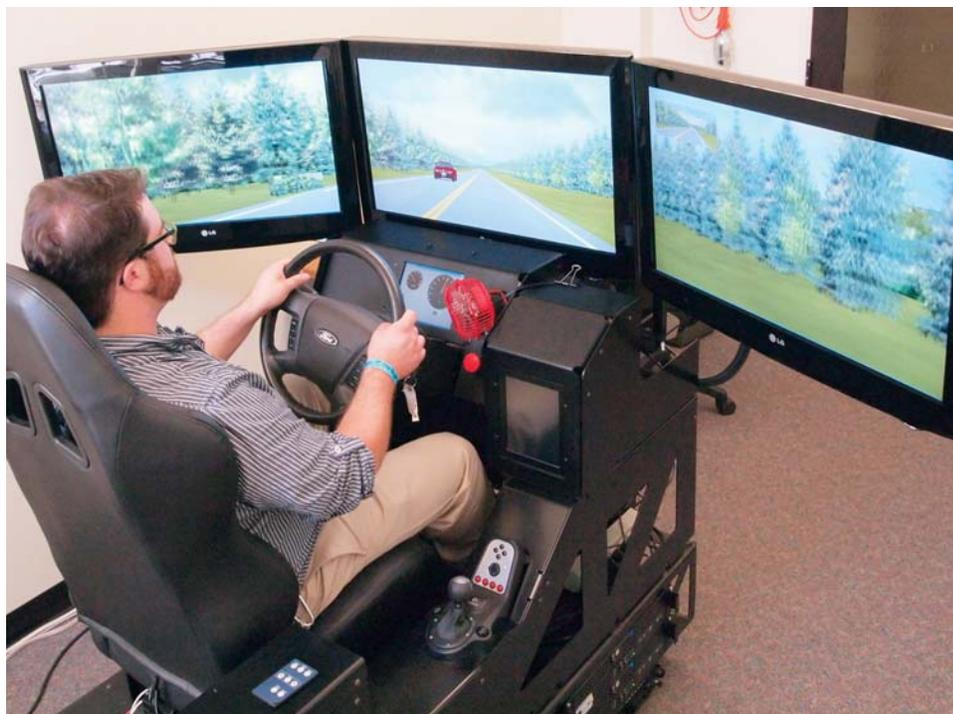
The HumanFIRST portable driving simulator is equipped with three 32-inch HD displays, mirror displays and vehicle controls.
