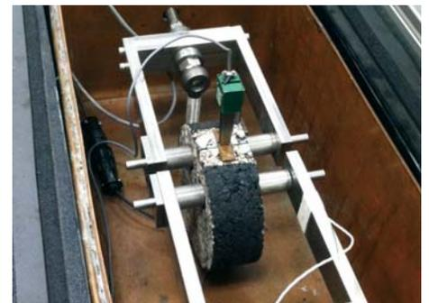
A disk-shaped asphalt sample held by clamps in a refrigerated box.
