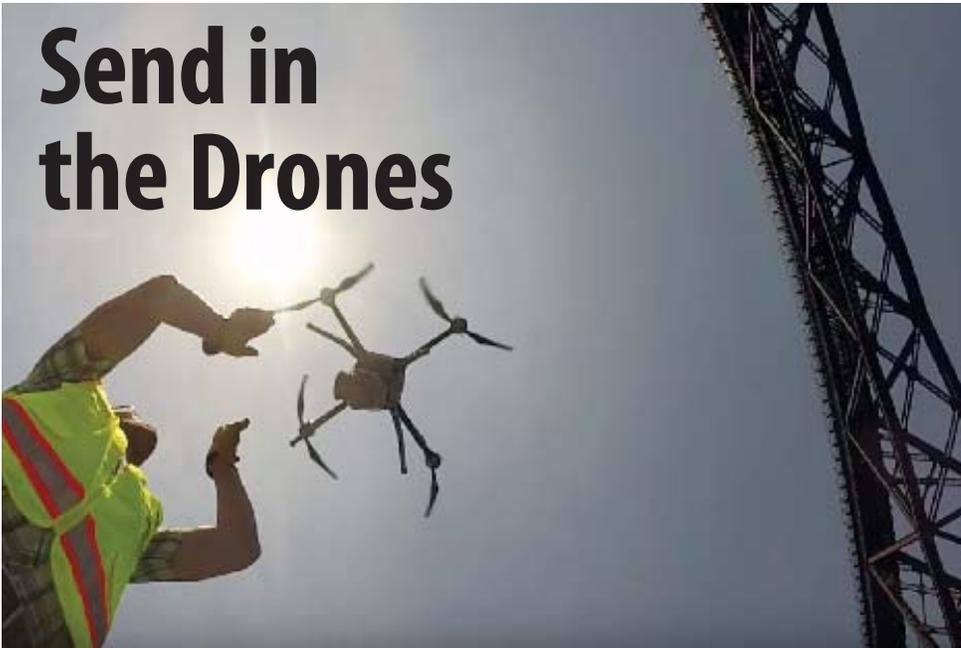
Bridge inspectors utilized the Aeryon SkyRanger drone, shown here, on four bridges after receiving FAA approval.
