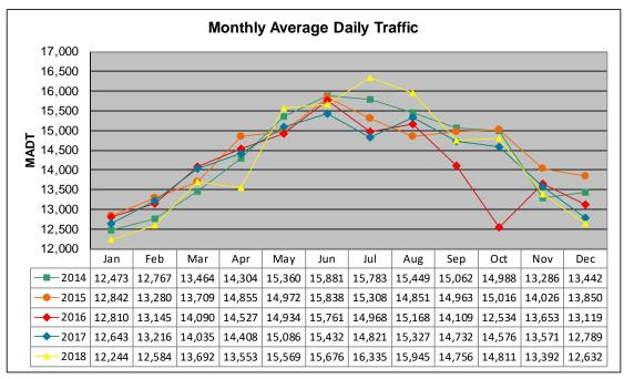
Note: Increase in traffic July/August 2018 due to detours... Decrease in traffic September/October 2016 due to construction on TH 12
