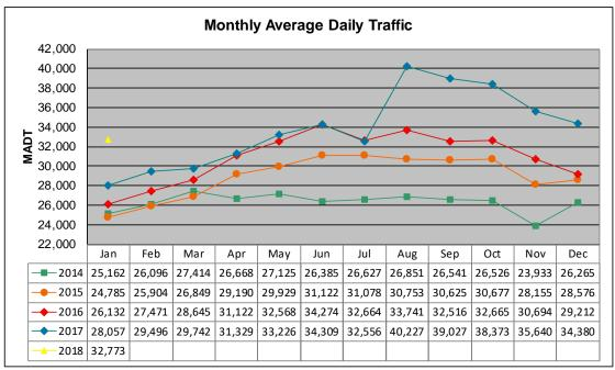
Note: Decrease in traffic April to November 2014, and May 2015 due to construction on TH 36... Increase in traffic beginning August 2017 due to completion of St. Croix Crossing Project on TH 36
