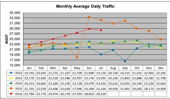
Note: Decrease in traffic Jul-Sep 2012 and May 2015 due to construction on TH 14... Increase in traffic beginning Nov 2012 due to an addition of two lanes at the site, and during Jun-Dec 2015 and Apr-Jul 2016 due to detours
