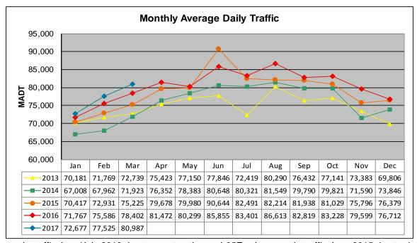
Note: Decrease in traffic June/July 2013 due to construction on I-35E... Increase in traffic June 2015 due to detour from MN 77
