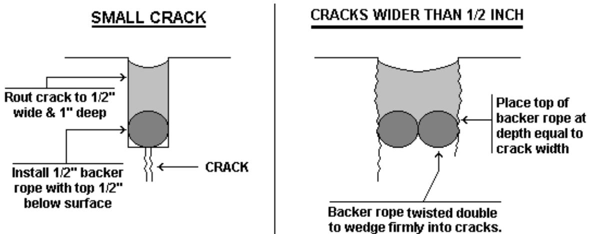
Figure 2. Crack sealing.
