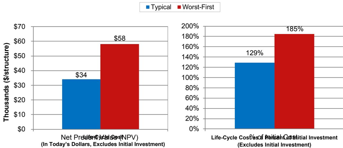
The results of the life-cycle cost analysis for high-mast light tower structures highlighting the magnitude of differences in costs for each strategy are shown in **Figure 6-13**.
