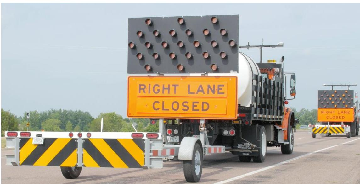
An ATMA truck follows the path of lead maintenance vehicles by using connected and automated vehicle technology. The lead vehicle leaves “electronic bread crumbs” for the ATMA to follow, allowing the ATMA to operate autonomously. For this project demonstration, a safety driver will be in the ATMA vehicle at all times. In the future, ATMAs have the potential to increase safety during mobile work zone operations by not needing a driver, keeping workers out of harm’s way.
