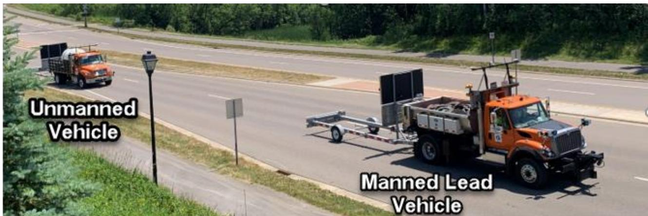
1. Retrofit existing MnDOT maintenance vehicle and install "ATMA kit" technology
