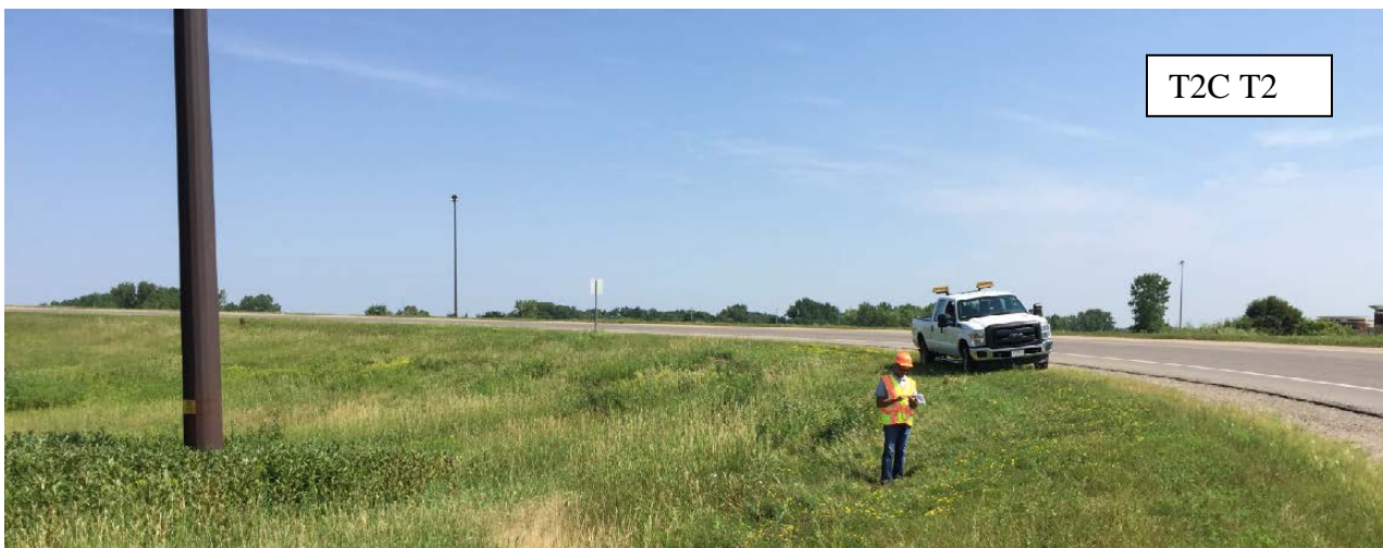
Figure 2: T2C T2 is located in the SE cloverleaf ramp with good sight distances and CPT truck access. This is the deepest existing foundation at the site and different than the estimated depths of the other two towers, making it a preferred location.
