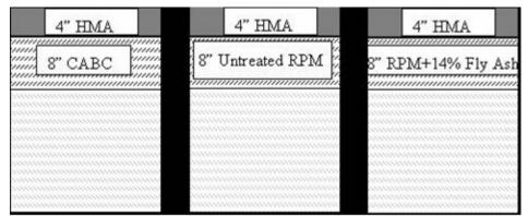
Pavement Structures of Test Sections at MnROAD
