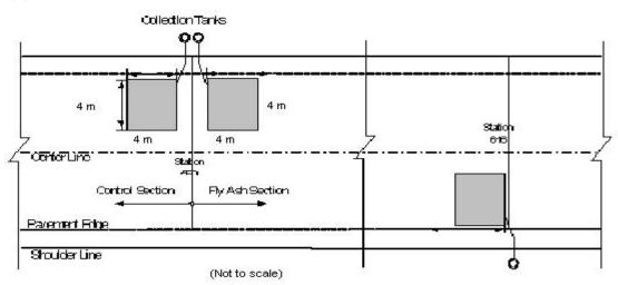
Fig. 1. MnROAD control and fly ash test sections: (a) profiles of pavement structure and (b) layout of three lysimeters.
