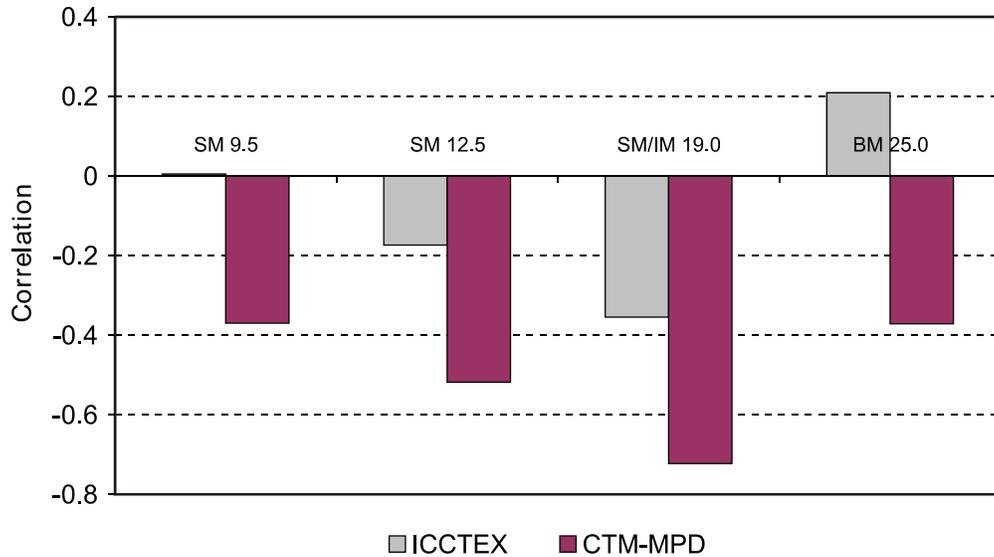
**Figure 1. Correlation of AC Content ( $P_b$ %) with Texture, All Mixes.** SM 9.5 = surface mix with 9.5 mm nominal maximum aggregate size (NMS). SM 12.5 = surface mix with 12.5 mm NMS. SM/IM 19.0 = surface/intermediate mix with 19.0 mm NMS. BM 25.0 = base mix with 25.0 mm NMS. CTM = circular track texture meter (ASTM E2157); CTM-MPD = CTM-based mean profile depth (MPD – ASTM E1845); ICCTEX = texture estimate from proprietary system developed by International Cybernetics Corporation.
