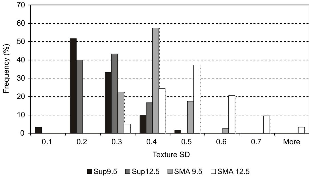
**Figure 5. Frequency distribution for texture fluctuation in the center of the lane.**
