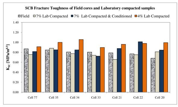
Figure 15. SCB fracture toughness test results for field cores
