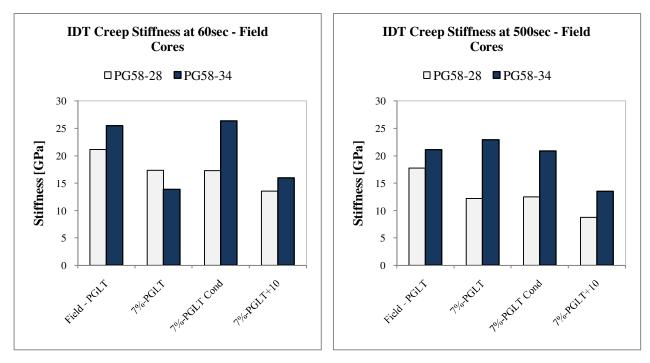
Figure 43. Effect of binder PG low limit on IDT creep stiffness
