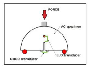
Figure 7. SCB test scheme
