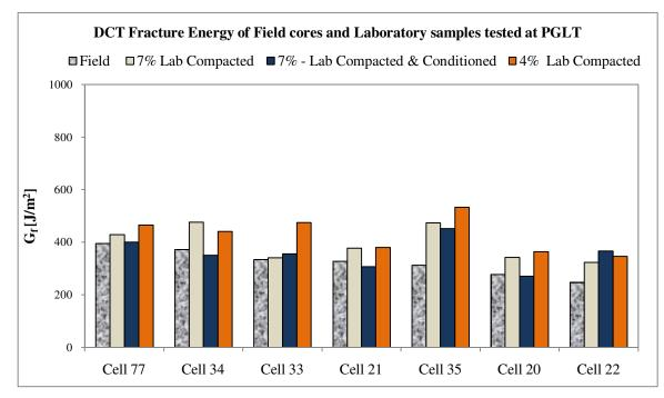
Figure 13. DCT fracture energy test results for field cores
