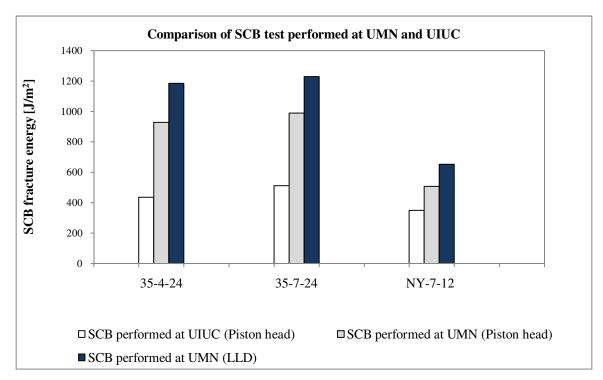
Figure 23a. SCB fracture energy from test performed at different laboratories
