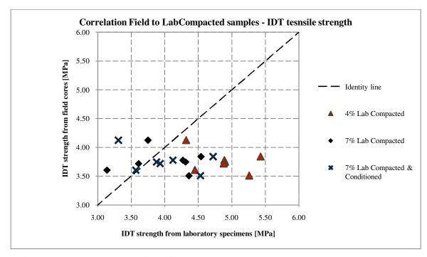
Figure 20. Results comparison field to laboratory compacted, IDT tensile strength
