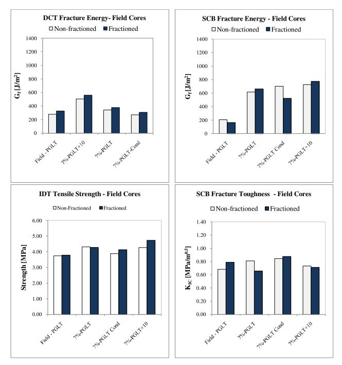
Figure 37. Effect of RAP fractioning on DCT, SCB, and IDT tensile strength -field
