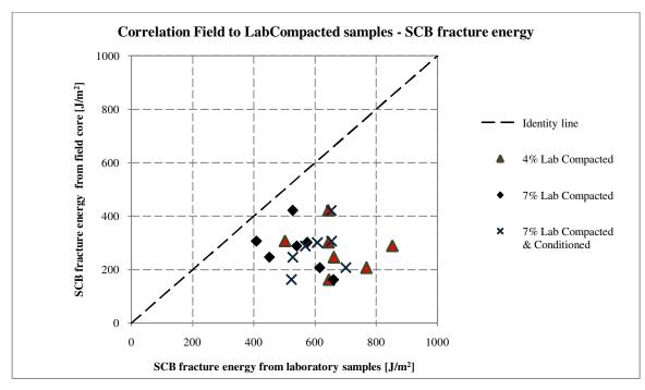
Figure 18. Results comparison field to laboratory compacted, SCB fracture energy
