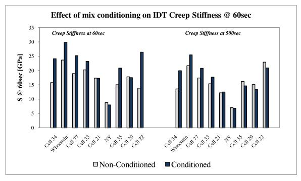
Figure 31. Effect of mix conditioning on IDT creep stiffness
