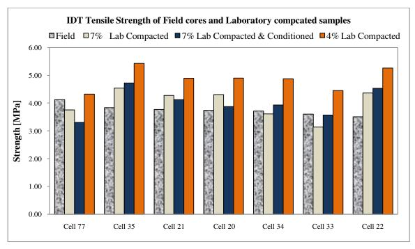
Figure 16. IDT tensile strength test results for field cores
