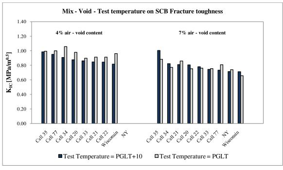
Figure 11. SCB fracture toughness test results
