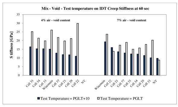
Figure 24. IDT creep stiffness at 60 sec test results
