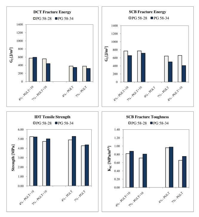
Figure 40. Effect of binder PG low limit on DCT, SCB, and IDT tensile strength
