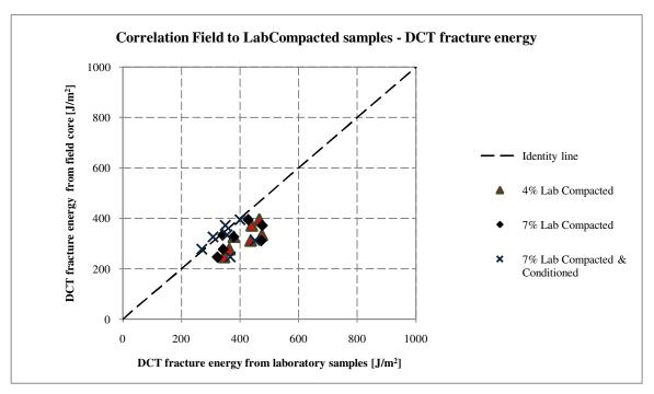
Figure 17. Results comparison field to laboratory compacted, DCT fracture energy
