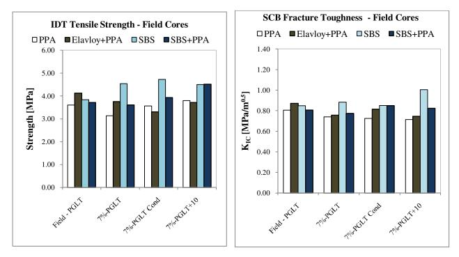
Figure 33. Effect of polymer and acid modifiers on DCT, SCB, and IDT strength - field
