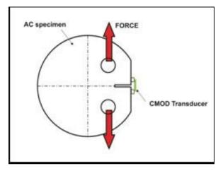
Figure 5. DCT test scheme
