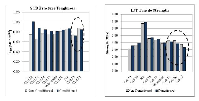
Figure 30. Effect of mix conditioning on DCT, SCB, and IDT tensile strength
