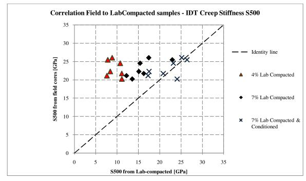
Figure 29. Results comparison field to laboratory compacted, IDT creep stiffness @ 500sec
