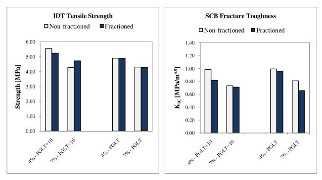
Figure 36. Effect of RAP fractioning on DCT, SCB, and IDT tensile strength
