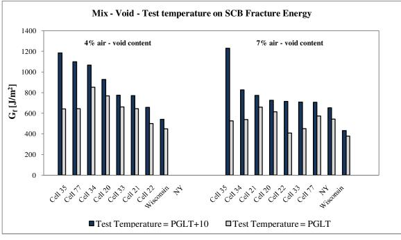
Figure 10. SCB fracture energy test results
