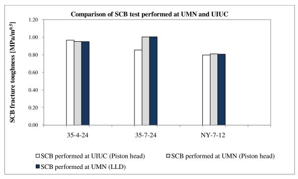
Figure 23b. SCB fracture toughness from test performed at different laboratories
