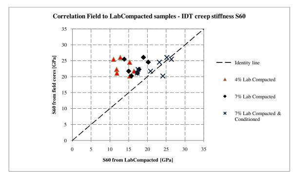
Figure 28. Results comparison field to laboratory compacted, IDT creep stiffness @ 60sec
