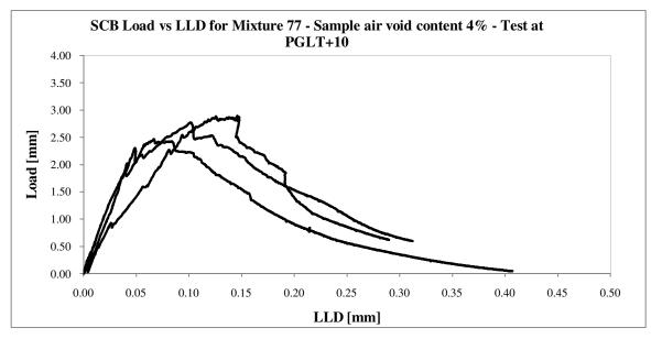
Figure 8. Typical Load-LLD plots from SCB tests of three replicates
