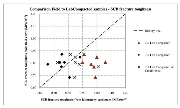
Figure 19. Results comparison field to laboratory compacted, SCB fracture toughness
