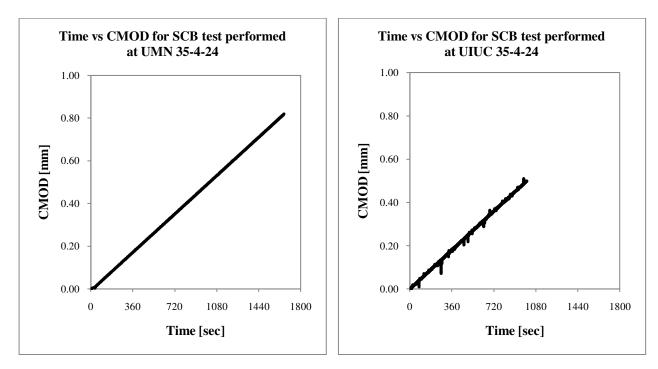
Figure 24. SCB fracture toughness from test performed at different laboratories
