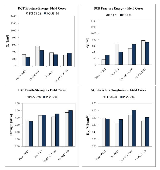
Figure 41. Effect of binder PG low limit on DCT, SCB, and IDT tensile strength -field
