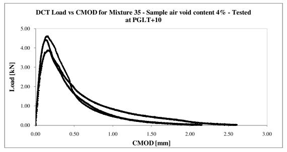
Figure 6. Typical Load-CMOD plots from DCT tests of three replicates
