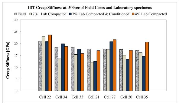
Figure 27. IDT creep stiffness at 500sec test results for field cores
