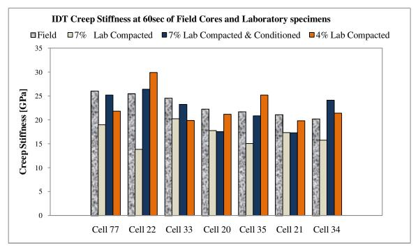
Figure 26. IDT creep stiffness at 60 sec test results for field cores
