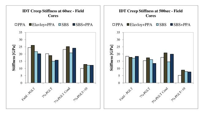
Figure 35. Effect of polymer and acid modifiers on IDT creep stiffness - field cores
