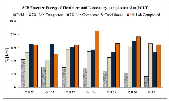
Figure 14. SCB fracture energy test results for field cores
