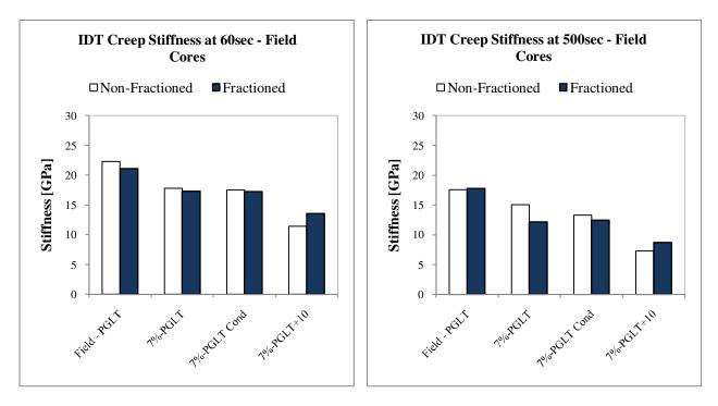
Figure 39. Effect of RAP fractioning on IDT creep stiffness -field
