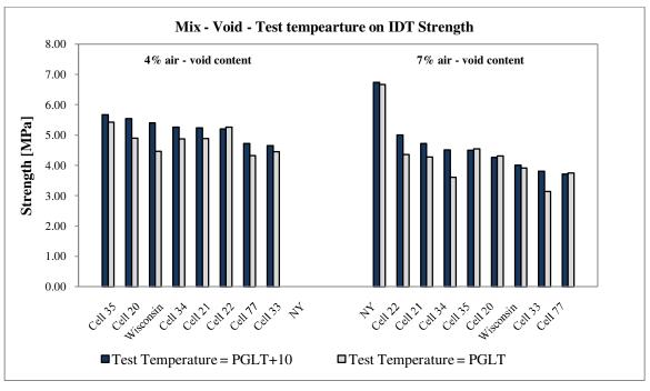
Figure 12. IDT tensile strength test results
