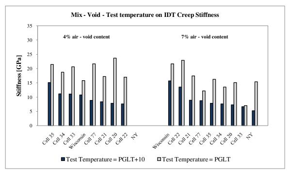
Figure 25. IDT creep stiffness at 500 sec test results
