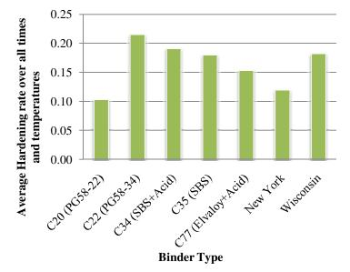
Figure 20: Comparison of the average hardening for each binder over all tested conditioning times and temperatures.
