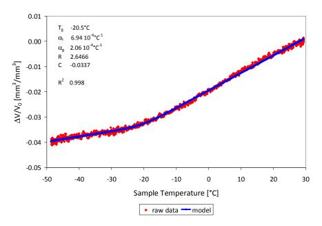
Figure 3: Typical results from glass transition temperature (T<sub>g</sub>) test of asphalt binders.
