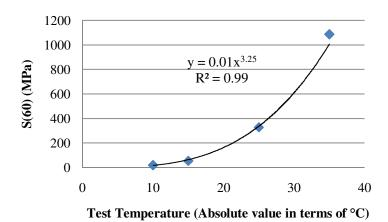
Figure 14: S(60) after 1 hr conditioning for one of the SHRP binders plotted against test temperature.
