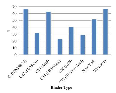
Figure 19: Comparison of the η parameter derived from the fitted physical hardening model.
