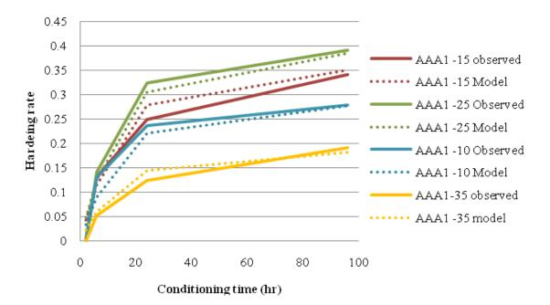
Figure 11: Comparison of model described by [4] with experimental data. (Hardening rate=  $\Delta S/S_0$ )
