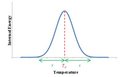
Figure 10: Empirical function used to account for glass transition temperature in prediction model. (2x is the length of the glass transition region)
