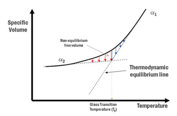
Figure 7: Schematic of proposed material behavior in glass transition region.
