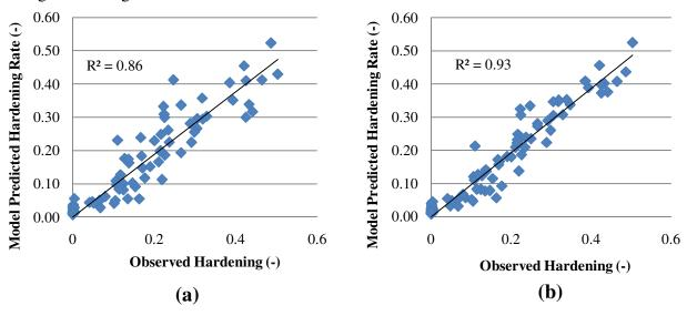
Figure 17: Goodness of fit of the physical hardening model for the MnROAD binders (a) using measured glass transition temperature values, (b) using values fitted by model.
