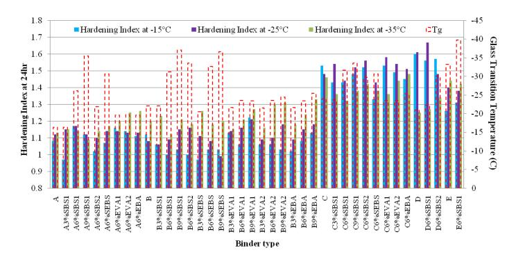
Figure 6: Hardening index after 24 hr of isothermal conditioning at different temperatures using data from Lu and Isacsson (5).
