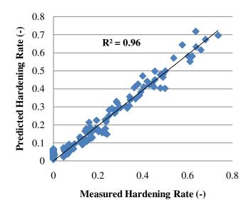
Figure 13: Goodness of fit between model described by [4] with fitted T<sub>0</sub> and experimental data. (Hardening rate=  $\Delta S/S_0$ )
