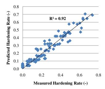
Figure 12: Goodness of fit between the predictions using Equation [4] using  $T_g$  for  $T_0$  and the experimental data. (Hardening rate=  $\Delta S/S_0$ )
