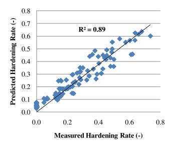
Figure 16: Goodness of fit between model described by [6] using  $T_g$  for  $T_0$  and experimental data.
