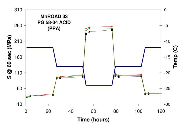
Figure 8: PG 58-34+ PPA binder from MnROAD 33- creep stiffness as function of conditioning time.
