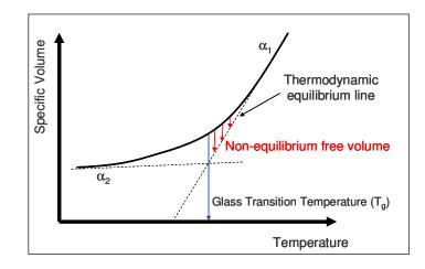
Figure 1: Physical hardening and its relation to free volume
