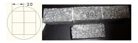
Figure 26: Prismatic beams made from gluing blocks cut out of gyratory samples.
