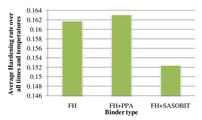
Figure 21: Comparison of the average hardening for each binder over all tested conditioning times and temperatures.
