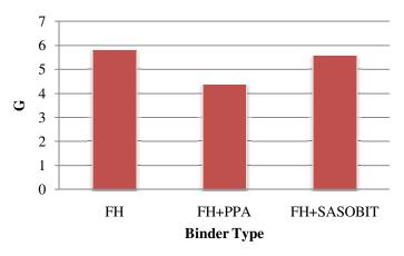
Figure 22: Comparison of G parameter derived from the fitted physical hardening model.
