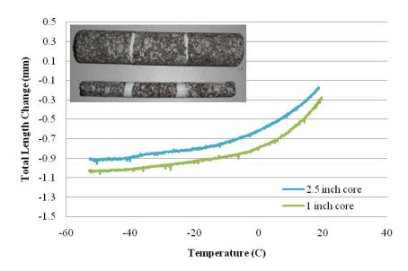
Figure 25: Comparison of  $T_g$  results from samples with  $\phi = 1''$  and 2.5''.
