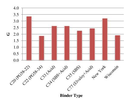
Figure 18: Comparison of the *G* parameter derived from the fitted physical hardening model.
