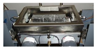
Figure 27: Test setup used for the glass transition temperature of beams made from gyratory compacted samples
