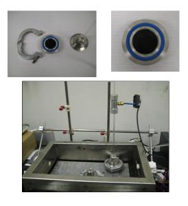
Figure 2: Dilatometric system used to measure glass transition temperature (T<sub>g</sub>) of asphalt binders.
