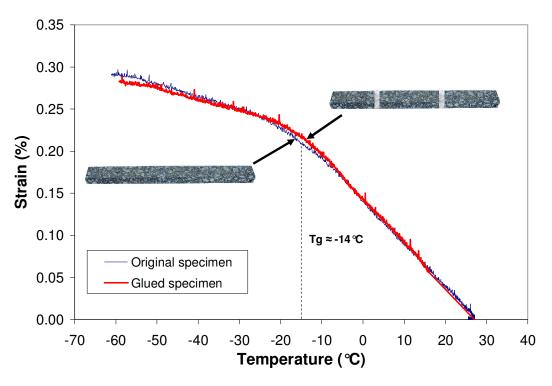
Figure 24: T<sub>g</sub> mixture results for unglued and glued specimen.
