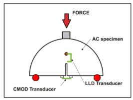
Figure 3. SCB testing scheme
