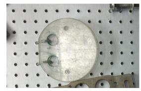
Figure 6. DC(T) marking template
