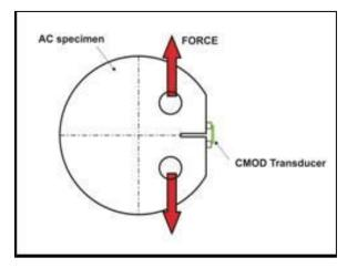
Figure 1. DC(T) testing scheme
