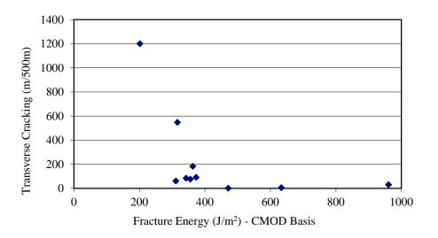
Figure 1. Field Data Suggesting a Minimum Fracture Energy of 400 J/m<sup>2</sup> at PGLT + 10°C to Prevent Thermal Cracking
