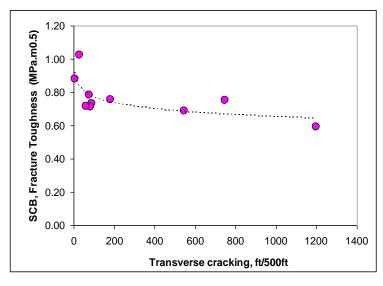
Figure 3. Field Data Suggesting a Minimum Fracture Toughness of 800kPa×m<sup>0.5</sup> at PGLT + 10°C to Prevent Thermal Cracking
