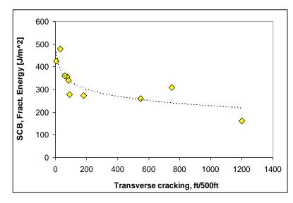
Figure 2. Field Data Suggesting a Minimum SCB Fracture Energy of 350 J/m<sup>2</sup> at PGLT + 10°C to Prevent Thermal Cracking
