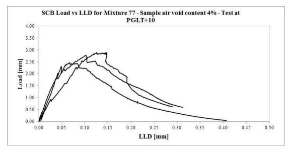
Figure 4. Typical Load-LLD plots from SCB tests of three replicates
