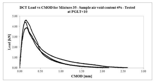
Figure 2. Typical Load-CMOD plots from DCT tests of three replicates
