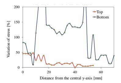
Figure 17. Variation of vertical stresses along the thickness of the measurement strip
