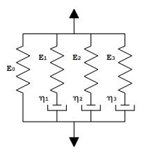
Figure 8. Generalized Maxwell Model (GMM)
