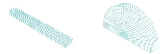
Figure 12. 3D model representations of 3-point bending and notched semi-circular beams
