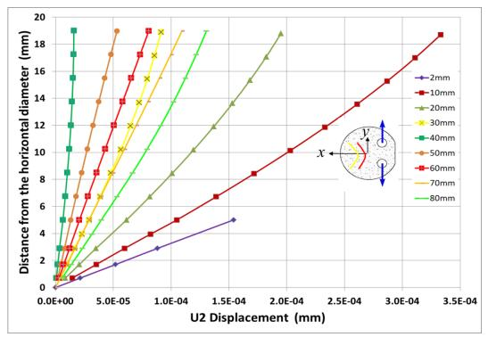
Figure 10. DCTIDT sample without Notch Elastic Simulation Results
