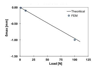
Figure 14. Calibration of the 3-point bending beam FE model
