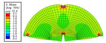
Figure 11. SCB stress state for a load of 1 kN
