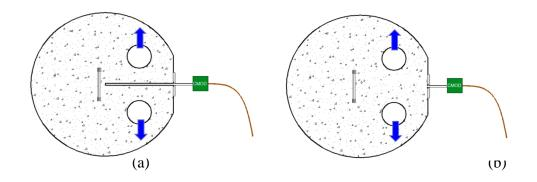
Figure 5. (a) DCTIDT sample with Notch (b) DCTIDT sample without Notch
