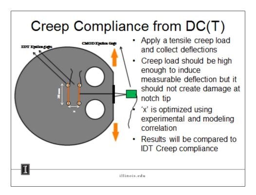
Figure 1. Concept of obtaining creep compliance from DC(T) test
