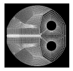
Figure 4. Finite Element Mesh of DCTIDT Sample
