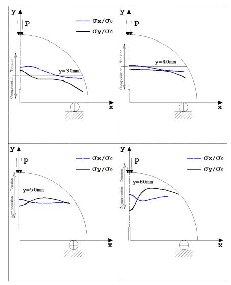
Figure 14. Stress distribution along several horizontal trajectories in SCB specimen
