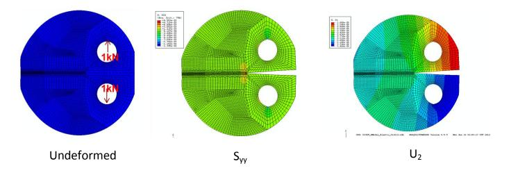
Figure 6. DCTIDT sample with Notch Elastic Model Simulation Results
