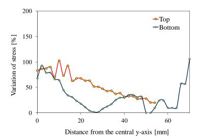
Figure 16. Variation of transversal stresses along the thickness of the measurement strip
