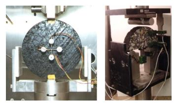
Figure 15. IDT and SCB experimental testing setup
