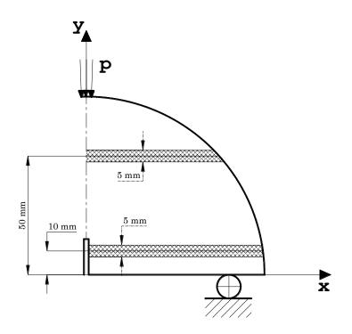
Figure 15. Potential SCB profiles for displacement measurements
