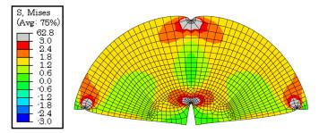
Figure 12. SCB stress state for a load of 2 kN
