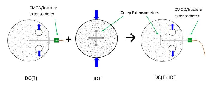
Figure 2. Comparison of Disk-shaped Compact Tension [DC(T)] test, Indirect Tension Test (IDT) and combined DC(T)-IDT test geometries.
