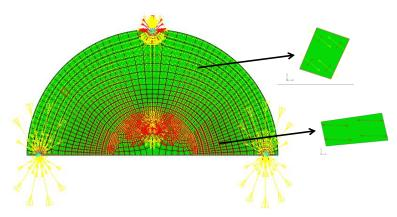
Figure 13. SCB stress state – plot of principal stress
