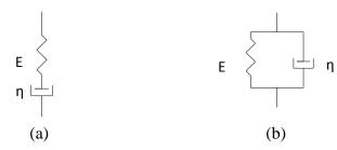
Figure 37. Maxwell Model (a) and Kelvin-Voigt Model (b)
