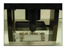
Figure 31. Bending Beam Rheometer with beam of asphalt mixture
