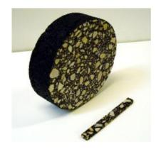
Figure 32. IDT and BBR test specimens
