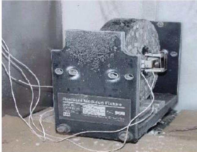
**Figure 8. Indirect Tensile Test Setup**
