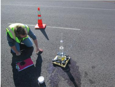
A researcher conducts an on-site permeability test to determine how well a pothole repair seals and resists water penetration.
